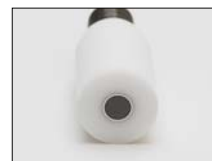
Figure 1. Rotating ring-disk electrode (RRDE). The ring electrode is kept at open circuit potential.
